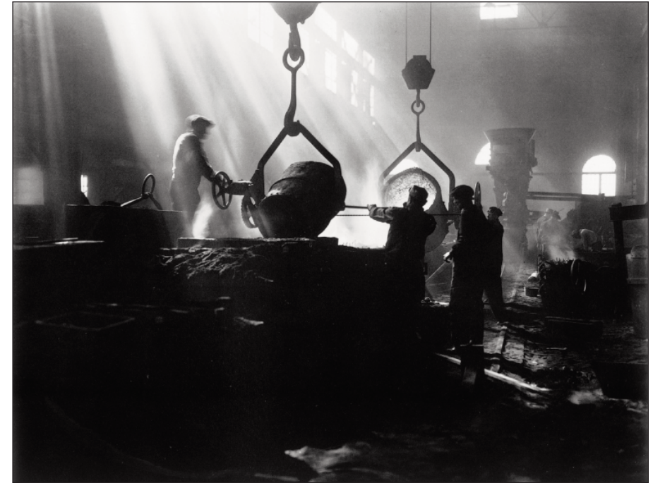
Filling Molds with Molten Iron I, 1934. Photograph by Luke Swank.
